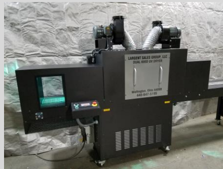
UV Dryers in DUAL bulb 400 WPI + 600 WPI. Dryers also available in rotary footprint + lab units .
