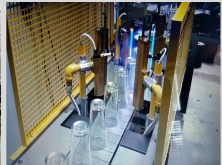
X-Pattern flame treat can be used in-line before PYROSIL, or in a modular conveyORIZED setting.
