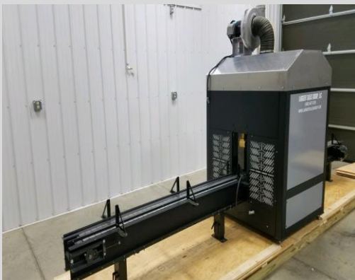
Pyrosil pre-treatment in-line to CNC without X-Pattern, nor (2) additional flame heads.
