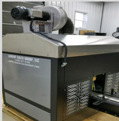
Pyrosil pre-treatment in-line to CNC without X-Pattern, nor (2) additional flame heads.
