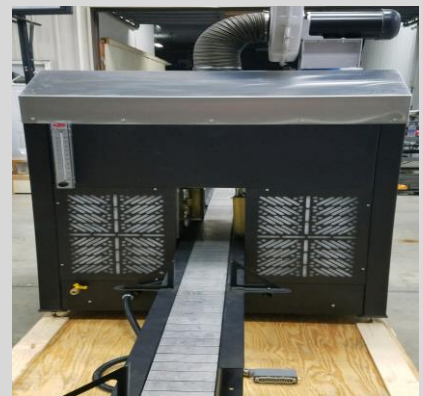
Pyrosil pre-treatment in-line to CNC without X-Pattern, nor (2) additional flame heads.
