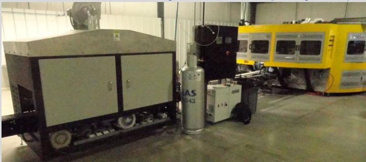
Bottle feeder, full X-Pattern, + Pyrosil dual burner system interfaced with CNC 6600L decorator.
