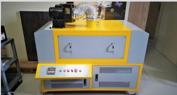
Basic DUAL UV Dryer 480V 3-phase
