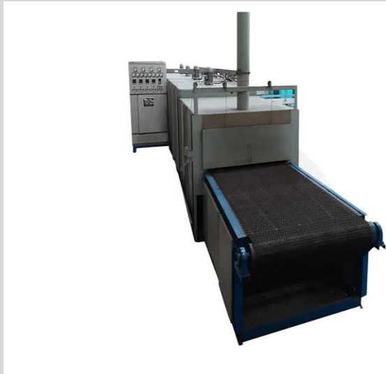
Model: LEHR - WLD-RK1200 Band Length: 24.4 Mts Belt Width: 1.20 Mts Electrical power supply: 3P 380V Machine dimensions: 24.5 Mts x 1.70 Mts Maximum temperature: 300°C Electric Lehr
